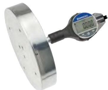
SmartPlug for large diameters (up to 280mm)
