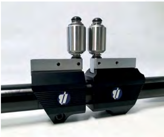
The Universal Gauge can also be used for thread measurement. Thread rolls would be formed to suit requirements.
